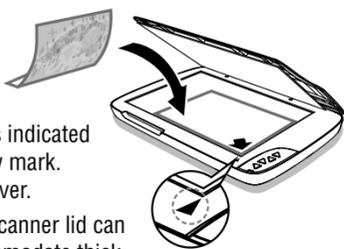
**Note:** The hinges of the scanner lid can extend upwards to accommodate thick items.
